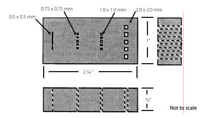
Figure 1-2. Resolution Block Detail
